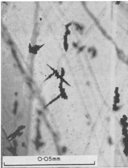
Figure 3 Included impurity dendrites in an YVAN crystal.
