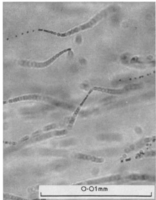
Figure 4 Wandering stringers of uniform size dendrites in YVAN.
