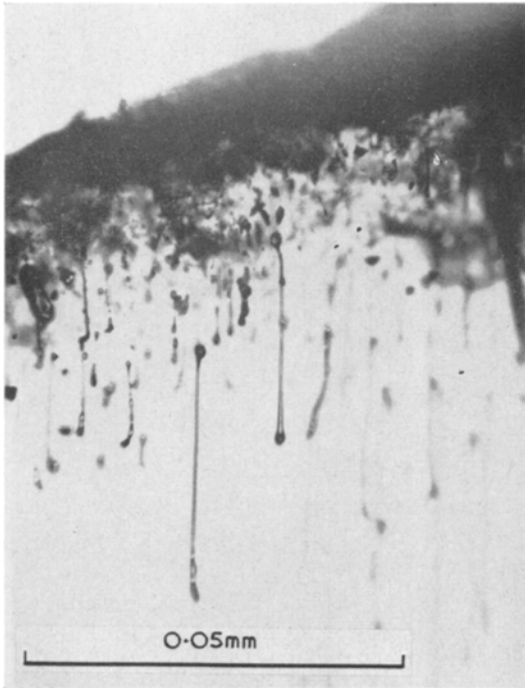
Figure 2 Bubble inclusions in YVO_4 .
